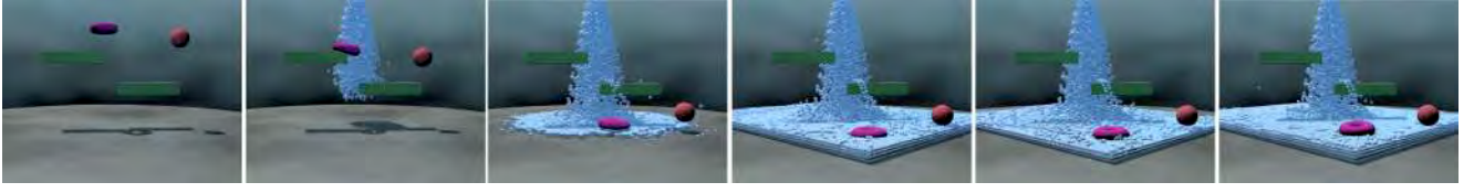
Fig. 16 A shower of fluids, which consists of 45K ISPH particles together with a lifebuoy and a ball of 35K PBD constraints. The lifebuoy and ball have different masses, and the lifebuoy is a bit heavier than the ball. While the fluid is filling a block volume, the ball floats, and the lifebuoy slowly rises to buoyancy.
